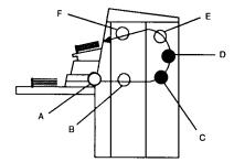
The sensors are located in the upper section of the lower roller assembly housing.
